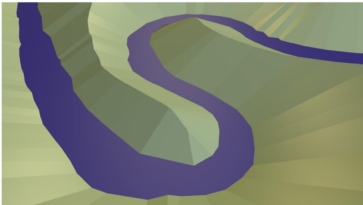
Figure 9: A terrain generated from the boundary of the blue river by our straight-skeleton implementation Bone. The figure illustrates the “Schlögner Schlinge”, which is a part of the river Danube in Austria (48°26' 10" N 13°51' 50" E). The boundary of the river is based on data obtained from OpenStreetMap [OSM].
